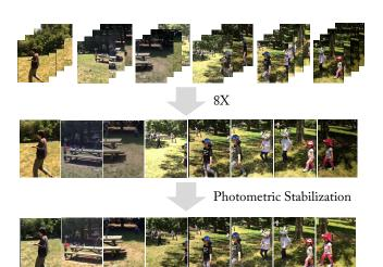
**Figure 1:** Photometric instability in fast-forward videos. (TOP) original image sequence with photometric jitter, e.g.brightness and tone fluctuations. (MIDDLE) sampled frames for fast-forward video with a speedup of 8, which exacerbates the photometric variations (BOTTOM) our result video after photometric stabilization.
