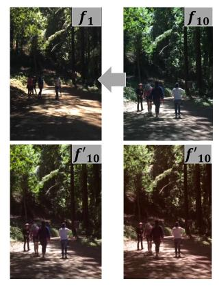
**Figure 2:** Color transfer by accumulating pairwise transformations. The reference frame is frame i and the target frame is frame i+10. The target is matched to the reference using accumulated transformation (in this case, the accumulation of 9 transformation matrices). (TOP) the reference and target frame pair (BOTTOM LEFT) the transformed frame with accumulation (BOTTOM RIGHT) the transformed frame with no accumulation.
