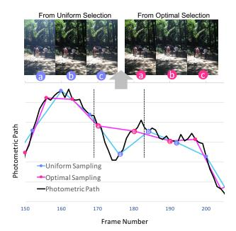
**Figure 5:** Uniform selection VS. optimal frame selection, which considers photometric constraints. The photometric path is computed using  $\bar{P}$  as described in Eq. (12). Note that the path from optimal selection avoids high frequency photometric change and is smoother than either the original or uniform selected paths. Shown on top, We can also visualize the frames being selected using uniform and optimal selection. The optimally selected frames are more photometrically consistent.
