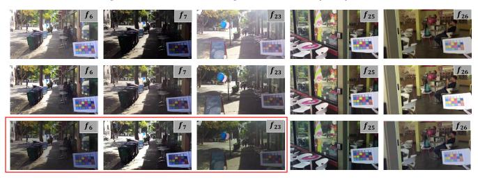
**Figure 11:** Experiment on a real video dataset. (TOP) input frame sequence; (MIDDLE) corrected frames using our method; (BOTTOM) corrected frames using Farbman et al. [FL11]. The input frame sequence contain brightness fluctuation due to the change from outdoor to indoor. Farbman et al. [FL11] fails to handle the over-exposed frame like  $f_{23}$ .
