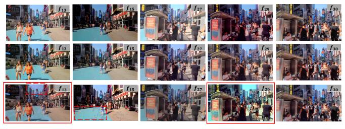
**Figure 7:** Synthetic experiment on outdoor scene dataset. (ROW 1) input sequence with brightness and color photometric instability (e.g.the  $2^{nd}$  and  $3^{rd}$  contain brightness jitter, and  $4^{th}$  frame contains color fluctuation); (ROW 2) stabilized frames using our stabilization method; (ROW 3) stabilized frames using Farbman et al. [FL11].
