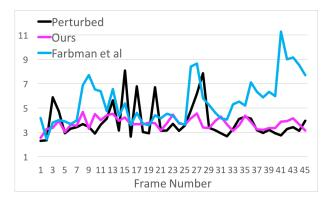
**Figure 8:** Quantitative evaluations on synthetic video experiments. We compute the RMSE for each frame, between the stabilized video and the ground truth video, and compared with Farbman et al. [FL11]. (LEFT) result on synthetic indoor scene, corresponds to Fig. 6 (RIGHT) result on synthetic outdoor scene, corresponds to Fig. 7.
