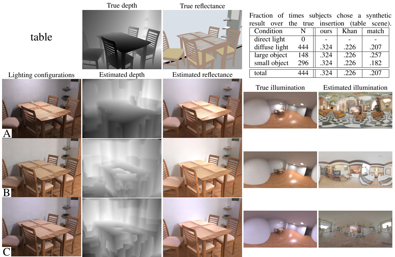
Fig. 15. Automatic scene estimates compared to the true depth, diffuse reflectance and illumination for the “table” scene.
